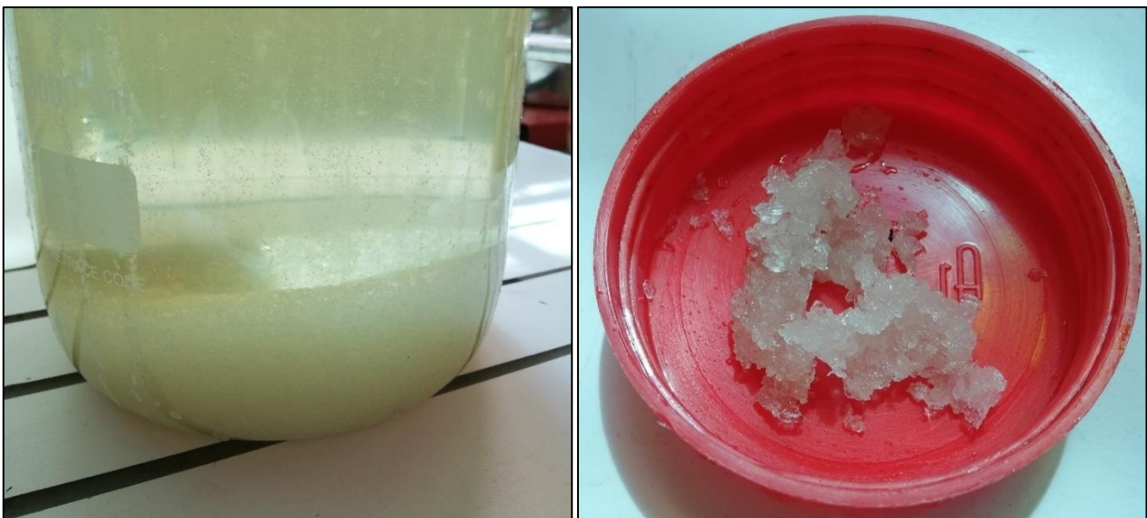
Figure 32. Ammonium sulphate precipitation due to overconcentration of ammonia in the sulfuric acid trap.
