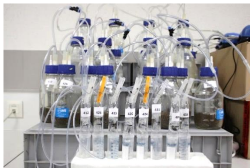
Figure 59. Experimental device for ammonia volatilisation (here, one block constituted of eight measurement chambers).
